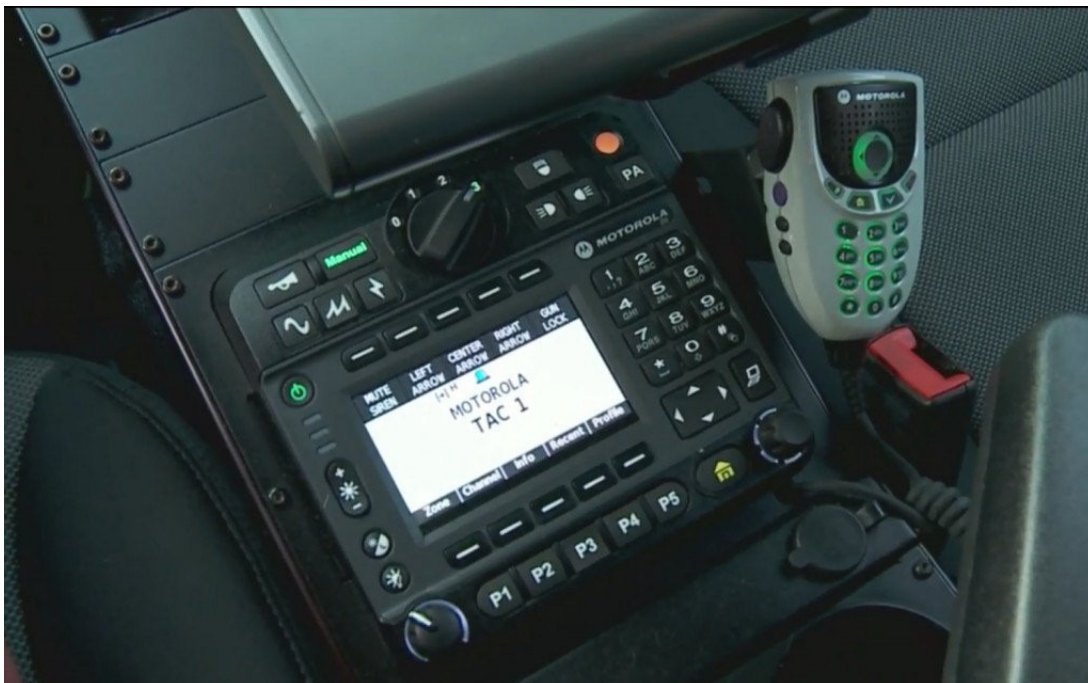
Figure G-1 Example of Center Console Mounting System
