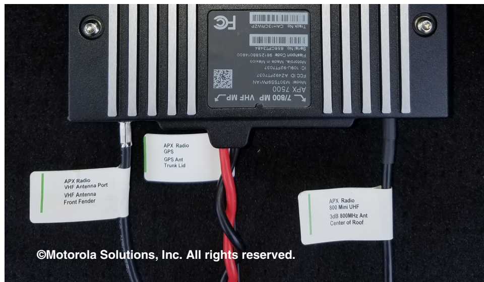
Figure G-8 Example of Coax Cable Labeling
