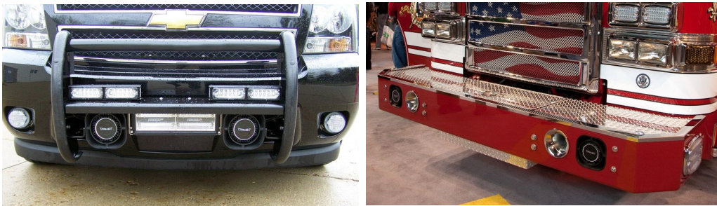
Figure G-41 Examples of Siren Installations (Photos Courtesy of Whelen®)
